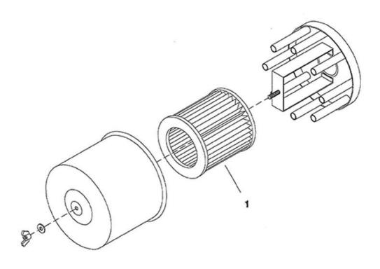
FIGURE 9. AIR INLET FILTER
