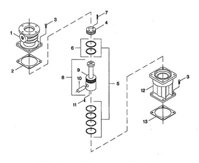
FIGURE 5. SECOND STAGE (3") PISTON. CYLINDER & CROSSHEAD
