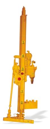
Pneumatic Slim Drill is designed for Marble and Granite mines for drilling in Down-The-Hole Hammer drilling method, ideally for drilling lead holes matching for Diamond Wire Cutting.
